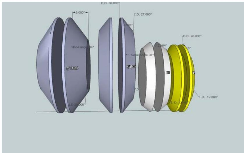
**Photo 1. Two new drill packer wheel assemblies under development at the WSU Dryland Research Station near Lind compared to existing technology. From left: 36-inch-tall with 6-inch-wide packer halves; 36-inch-tall with 4-inch-wide packer halves; 27-inch-tall International 150 packer assembly and; 26-inch-tall John Deere HZ packer assembly.**
