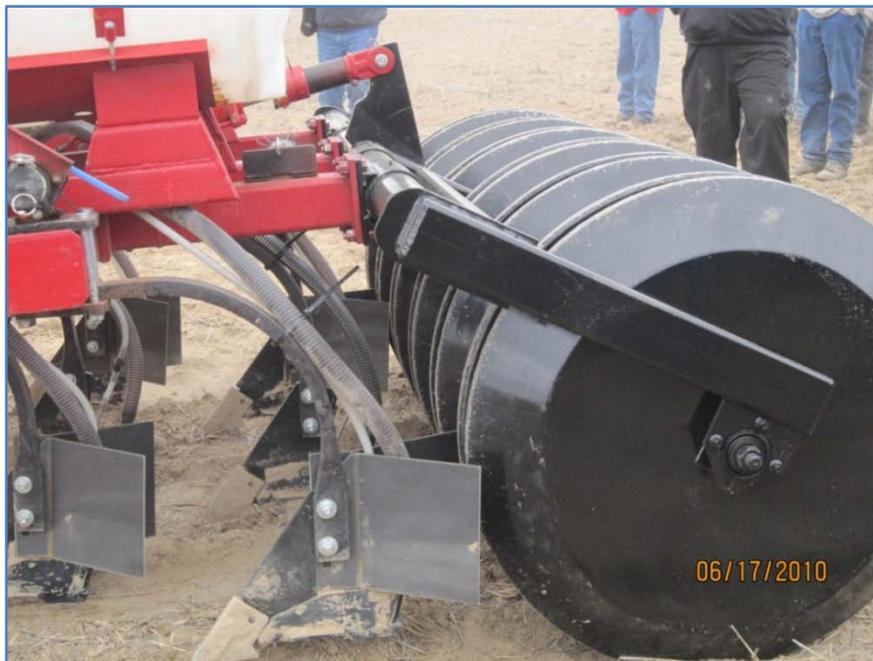
**Photo 2. One of the WSU Lind Station prototype deep-furrow drills with staggered shovel-type openers and 36-inch-tall packer wheels.**
