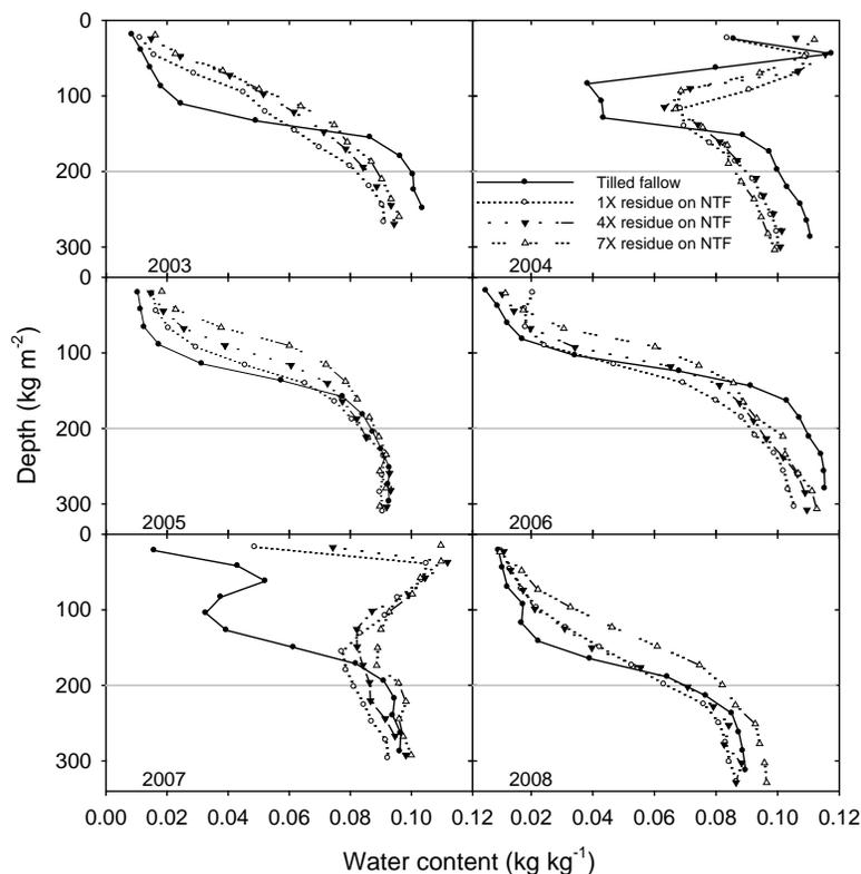
**Fig. 6. Seed-zone water content profiles measured in late August from 2003 to 2008 at Lind, WA. Samples were taken in 2-cm increments from 0- to 26-cm depth (22 cm in 2003) and are plotted on a dry soil mass per area basis in both tilled fallow and in no-till fallow (NTF) with three surface residue rates. The horizontal guideline marks 200 kg m<sup>-2</sup> used for equivalent-mass treatment comparisons.**
