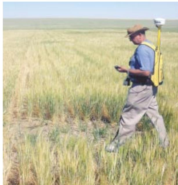
**Photo 5.** The surface areas of bare patches in the entire 20-acre experiment were measured each year using a backpack-mounted global positioning system.
