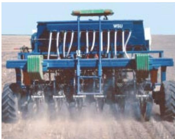
**Photo 3.** A Cross-slot notched-coulter no-till drill with 8-inch row spacing was used to plant all crops.
