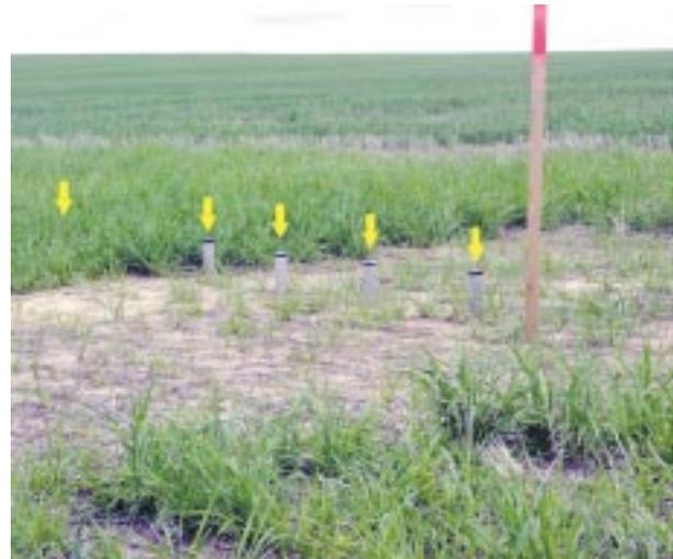
**Photo 4.** Neutron probe access tubes were installed in Rhizoctonia bare patches and healthy wheat to measure soil water content. Soil water levels were higher in bare patches, indicating that wheat roots do not grow into/ underneath bare patch areas.
