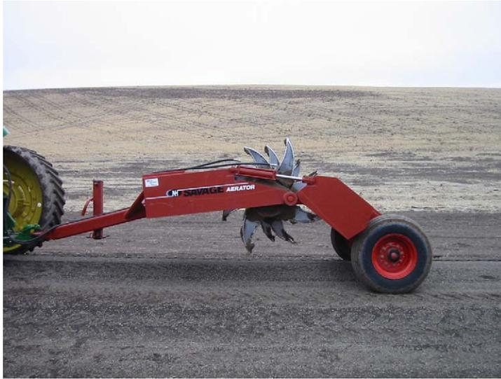
Fig. 2. Rotary subsoiler in transport position.
