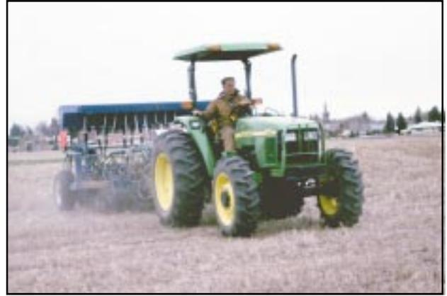
**Photos 2a and b. A Cross-slot TM disc drill with 8 in row spacing was used to simultaneously deliver seed and fertilizer in one pass through both CT (left) and NT (right) plots. Excellent stands of spring-sown wheat, barley, and oat were achieved in all 4 Y in both CT and NT plots.**
