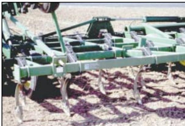
**Photo 1.** A duck-foot cultivator was used to prepare the seedbed in the CT plots. Two passes were made with the cultivator at a depth of 3 in.
