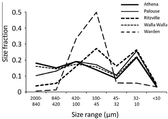
Fig. 4. Dry aggregate size distribution that characterized five soils for assessing threshold friction velocity inside a wind tunnel.
