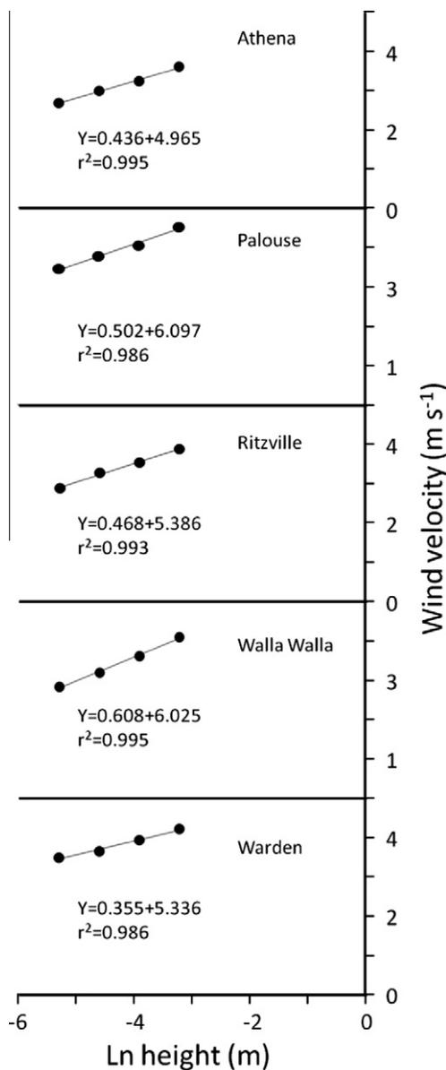
Fig. 2. Wind velocity as a function of the natural log of height above the surface of five soils. These data were collected inside a wind tunnel and used to assess friction velocity.
