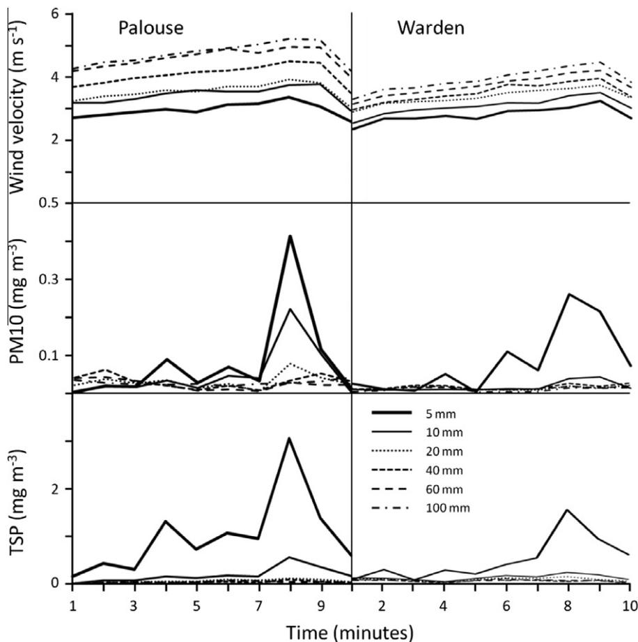
Fig. 5. One-minute time averages of wind velocity and PM10 and TSP concentrations at various heights above a Palouse silt loam and Warden silt loam inside a wind tunnel.
