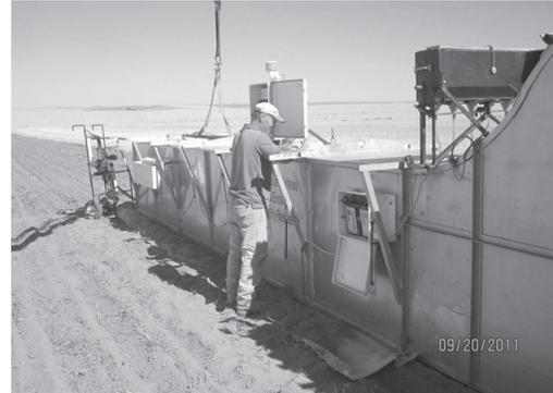
Fig. 1. A portable wind tunnel was used to measure soil sediment flux and PM<sub>10</sub> emissions, shown here at the Ron Jirava farm near Ritzville.
