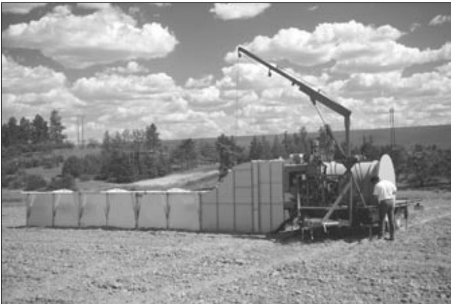
Figure 3.4. The portable wind tunnel designed by the  $CP_3$  has been utilized in much of the wind erosion prediction research on the Columbia Plateau. The machine generates variable wind speeds and simultaneously measures eroding soil including PM size that drifts through a 3.2 x 3.9 x 23.9 ft long rectangular tunnel. It is used to test the effect of soil and cover conditions on erosion loss for different wind speeds and soil types. Source: J.F. Kjelgaard, WSU.
