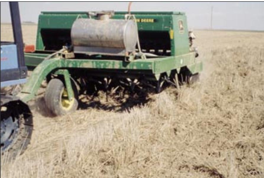
FIGURE 4.9. John Deere 9400 Series hoe drill used to sow the spring crop systems in the Ralston, WA field study. The drill though not specifically designed for no-till has performed well sowing into spring cereal stubble in terms of crop stands and range of residue levels. Photograph by F.L. Young, USDA/ARS, Pullman, WA.
